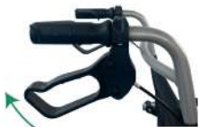
Image 1. To temporarily brake the chair, press the brake lightly. To advance, release the brake.
