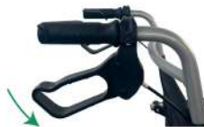
Image 2. To activate the locking system, press the brake down. To unlock it, lift the brakes upwards and you can continue to drive.
