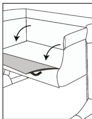
3. Lower the front panel by folding it down from both sides at the same time.
