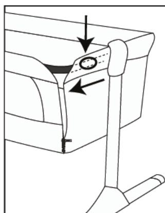
2. Locate the buttons under the fabric (where indicated by the circle), press them and remove the tube.
