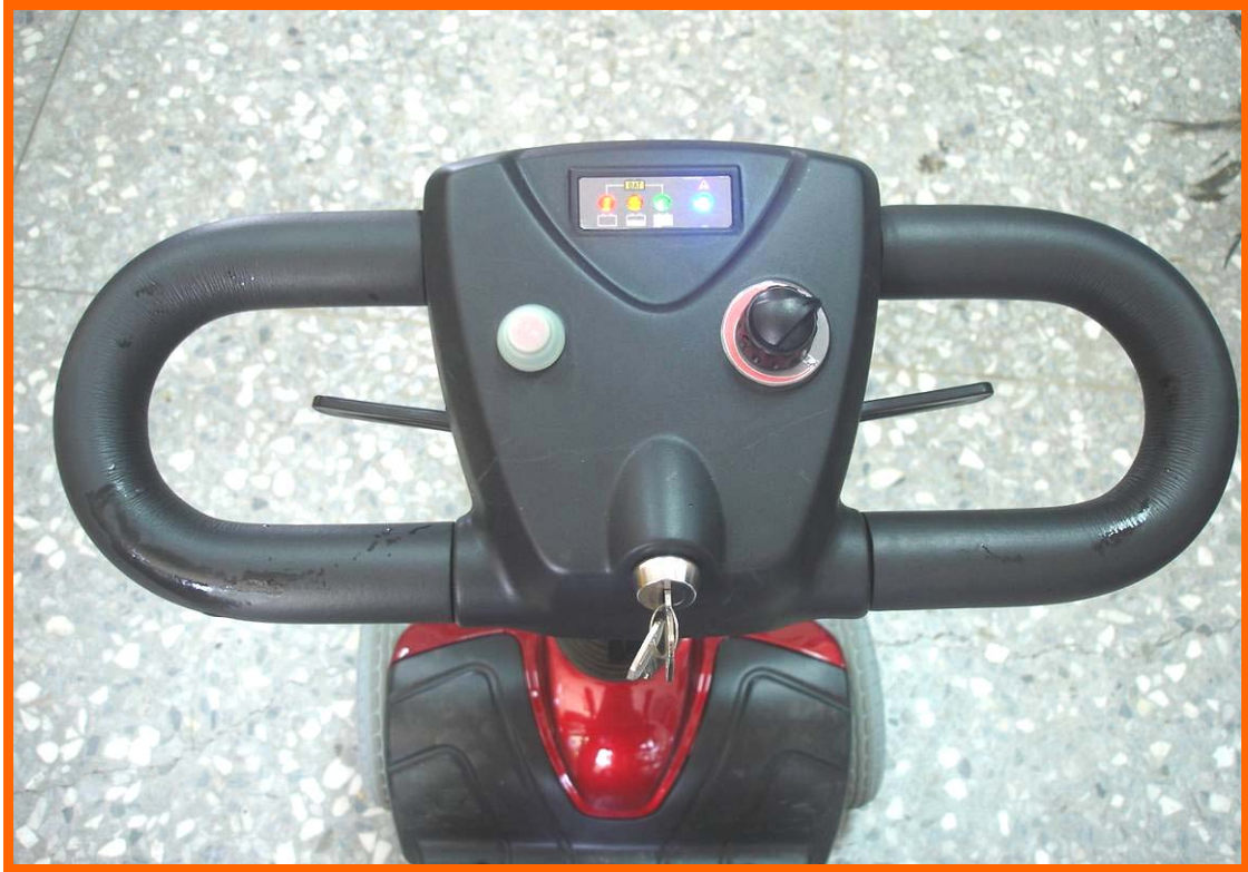
Photo 3 Top Control Panel view
